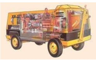
This industrial compressor uses compressed air to power heavyduty construction tools. Compressors are used for jobs, such as breaking up concrete or paving, drilling, pile driving, sandblasting and tunnelling. A compressor works on the same principle as a pump. A piston moves backwards and forwards inside a hollow cylinder, which compresses the air and forces it into a hollow chamber. A pipe or hose connected to the chamber channels the compressed air to the tools.
