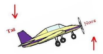
Case (ii): PROPELLER rotates in CLOCKWISE direction when seen from rear end and Aeroplane turns towards RIGHT
