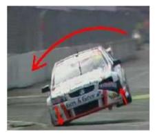
Due to the centrifugal couple, vertical reactions on the road surface will be produced. The reaction will be vertically upwords on the outer wheels and vertically downwords on the inner wheels. Let the magnitude of this reaction at the two outer and inner wheels be F Newtons, then,
