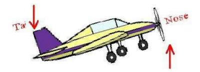
Case (v): PROPELLER rotates in CLOCKWISE direction when seen from rear end and Aeroplane takes off or nose move upwards
